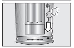
Remove the cappuccinatore from the steam and hot water spout by pulling it downwards.
